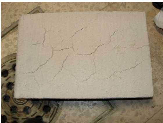
Figure 5 - Mortar prepared with quicklime pieces, QM.1-7 (7-day maturation)
