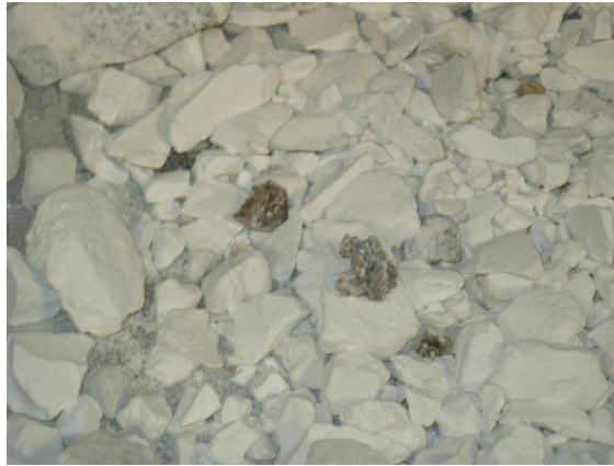
Figure 1 - Darker impurities in the industrial quicklime in stone
